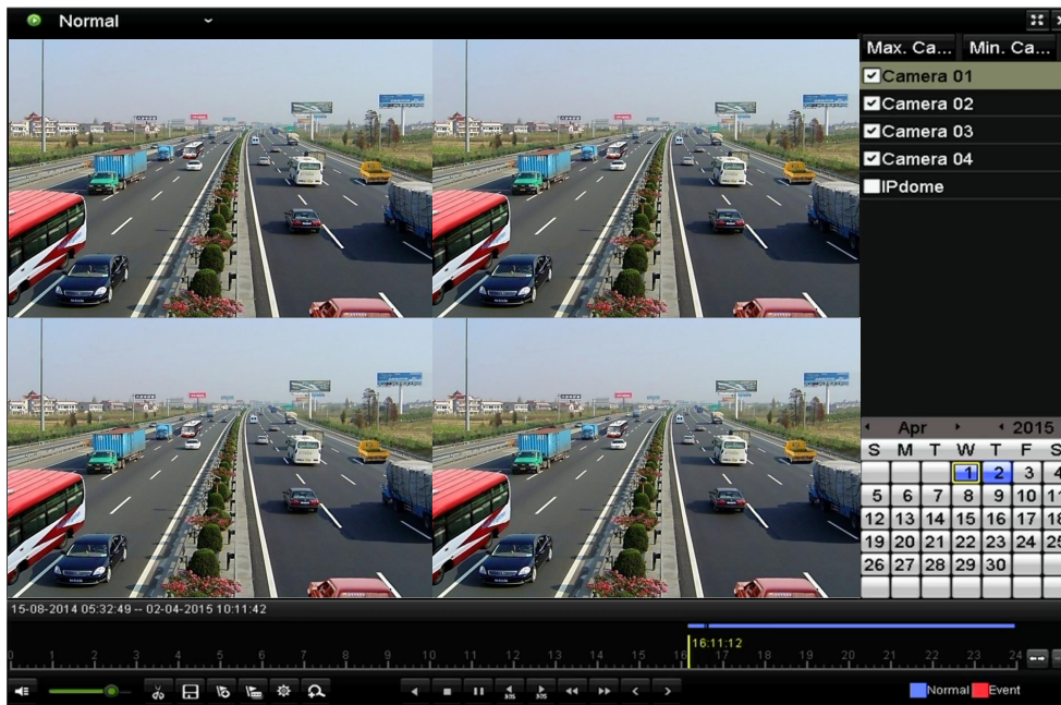
Figure 6. 19 4-ch Synchronous Playback Interface
